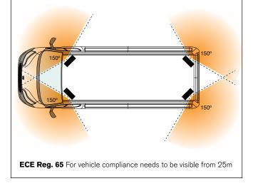
**Product Code RCV2217** Fixing Bracket or surface mount Operating voltage 10-30V DC 18W Maximum wattage Maximum current draw 1.5A @ 12V, 0.75A @ 24V Weight Lamp 196g, Bracket 70g Certification ECE R65, ECE R10 Number of LEDs 6 x 3W Flash patterns 10 Water proof IP67 Housing and lens Polycarbonate -40°C to 65°C Operating temperature Cable length 30cm Barcode 5055175246468
